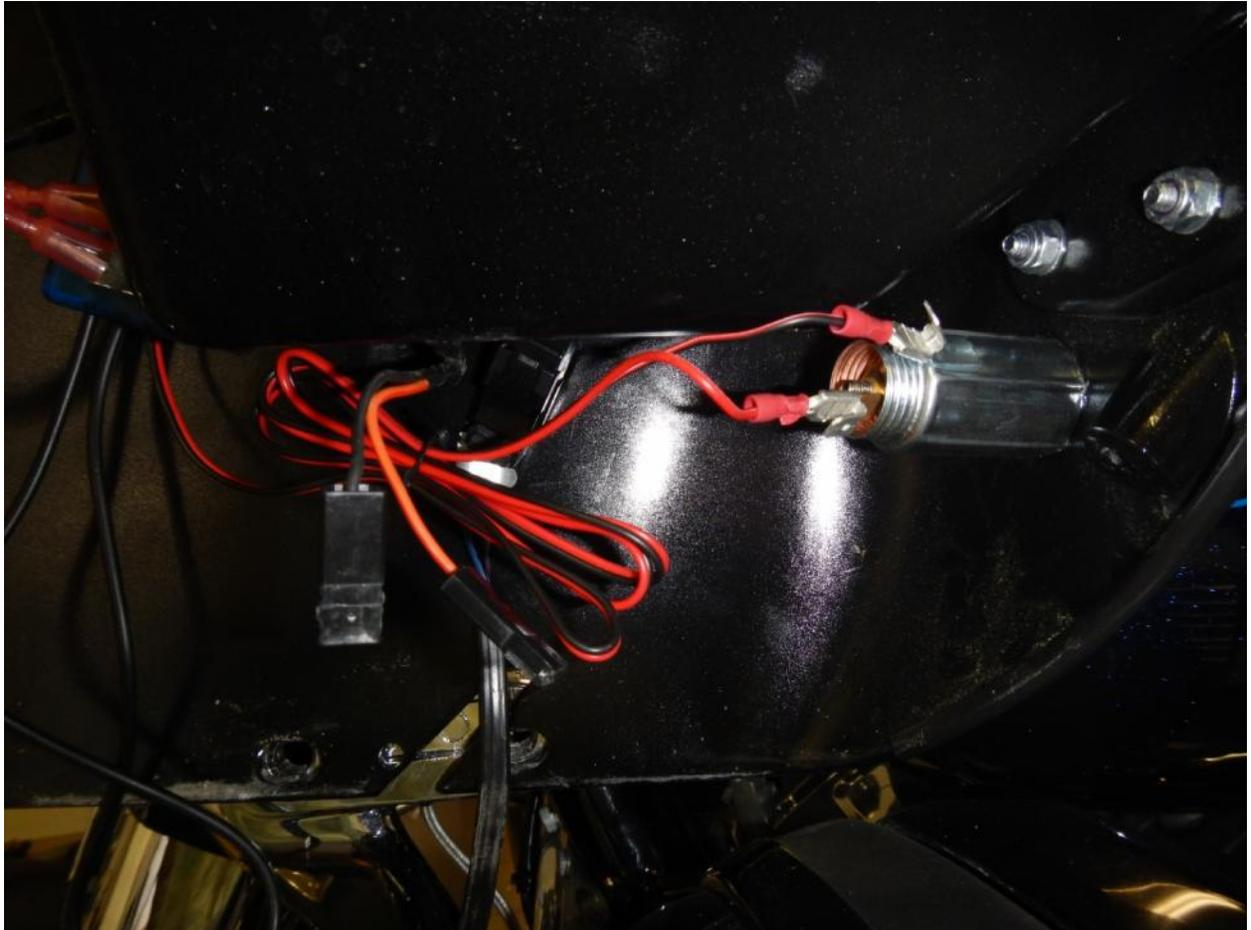
Plug the original wires into the BT-100M piggy back connectors. Our black wire connects with the stock black wire. Our red wire connects with the stock orange/white wire. Use the supplied wire ties to strap excess wire out of the way.
