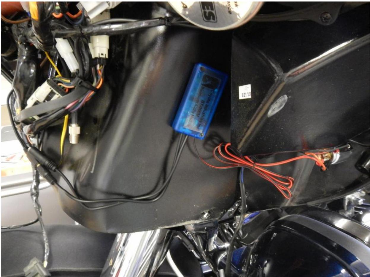
Route the power cable across and down to the back of the cigarette lighter. Remove the wires from the cigarette lighter and plug the wires from the BT-100M in their place. Our red wire goes to the center post. The black wire goes to the shell.
